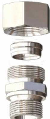
The Fluid Controls® DIN Connector is a three piece connector consisting of a Nut, Progressive Ring (ferrule) and Body. The progressive ring is case hardened by a **proprietary patented process** and the edge of the ferrule bites into the tube. This “biting” or “crimping” action is the heart of the connector and is a combination of geometry and metallurgy.
